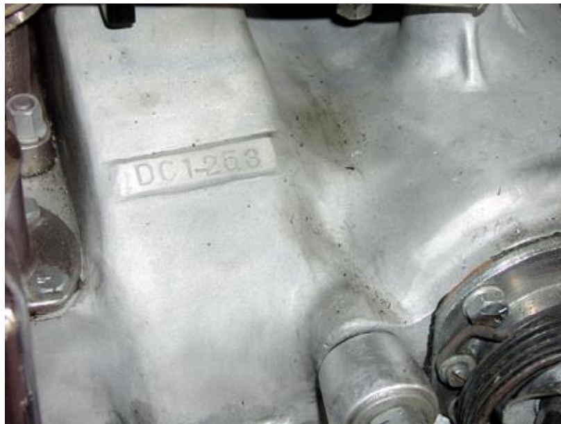
A top view of the finished product. This is the block that was not capable of being fixed. Can you see the inserted piece or the welds?
